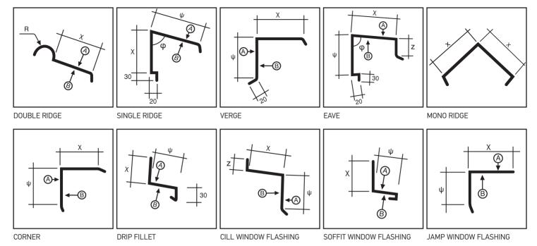
A wide range of flashing in different shapes, thickness and dimension are available under request.
